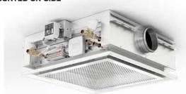
The room controller is factory mounted on the short side of LYRA II and wired. This configuration uses an external temperature sensor installed below the coil. Temperature and condensation (in option) sensor are factory wired.
